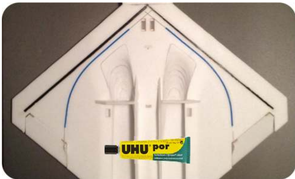
Pushrods made with z bends and sheathes glued using uhu POR (before fully set) - Also Foam safe CA may work (untested)
